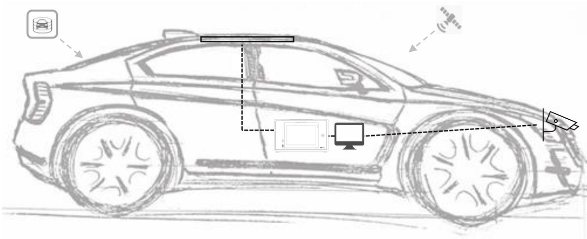
SPIDer™ set up: computer with SPIDer application, Magee Scientific Aethalometer® AE43, battery, CO2 sensor, cyclone, GPS, inlet, Smart-EYE.
