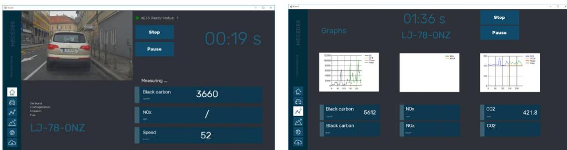
SPIDer™ application: during measurement Smart-EYE recognizes the license plate and retrieves relevant vehicle information (left). Real-time display of Black Carbon and CO2 concentration for emission factor determination.
