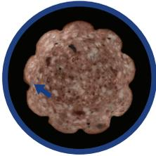
AnaliticaLabs.Vis4Q Wrapping Foil Detector uses **multi-spectral imaging technology (MSI)** to detect flakes of plastic wrapping foil, bones, cartilage and fat lumps in meat products with high resolution and **rapid detection speed**. Due to the nature of the technology, the objects of detection must be visibly exposed on the objects' surfaces or be detectable by light transmission.
